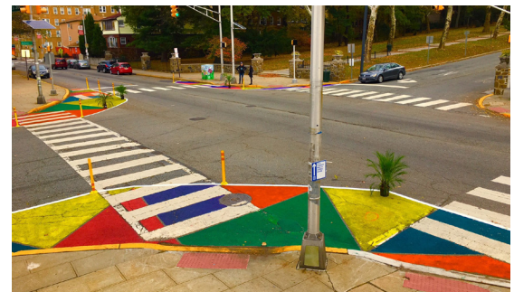
Painted curb extension and flexible delineators can be installed during the pilot project phase
